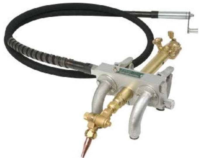
Manual transmission with torch
