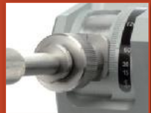
Eccentric plate triples the use of the diamond wheel.
