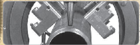
1SA Saddle Machine shown on 3" (76 mm) pipe
