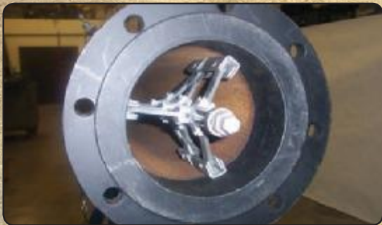
The 8" (203 mm) Internal Flange Alignment centers the ID of the 8" (203 mm) pipe to the ID of the flange for tack welding.
