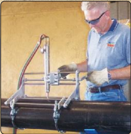
An excellent tool for making coupons for bend, tensile strength, and hardness tests.
